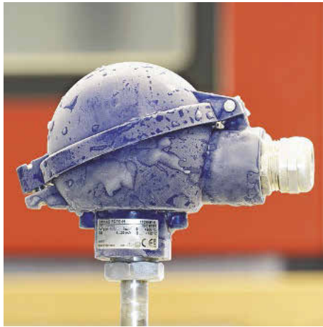
The instruments are cooled to -70\text{ }^{\circ}\text{C} in special climatic test chambers
